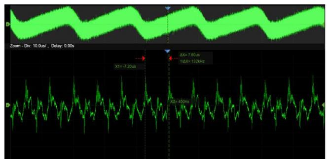
Using hardware-based Zoom technique and record length of up to 2.5 Gpts, users can select a slower timebase without compromising the sample rate, and then quickly zoom in to focus on the area of interest
