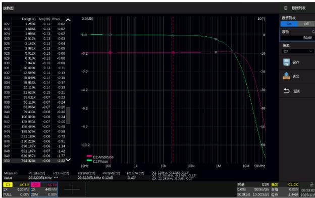
The oscilloscope can control the SIGLENT isolated USB AWG module or a stand-alone SIGLENT SDG generator, to scan the amplitude and phase-frequency response of the DUT, and display the data as a Bode Plot. This makes it possible to replace expensive network analyzers in some applications
