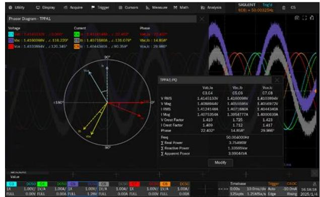
The Power Analysis and TPPA (3-phase Power Analysis) options provides a full suite of power measurements and analysis, which greatly improve the measurement efficiency in switching power supplies and power devices design. Combining the TPPA option with the 6/8 channels oscilloscope, high-voltage differential probes and current probes, we provide a complete solution of 3-phase power analysis
