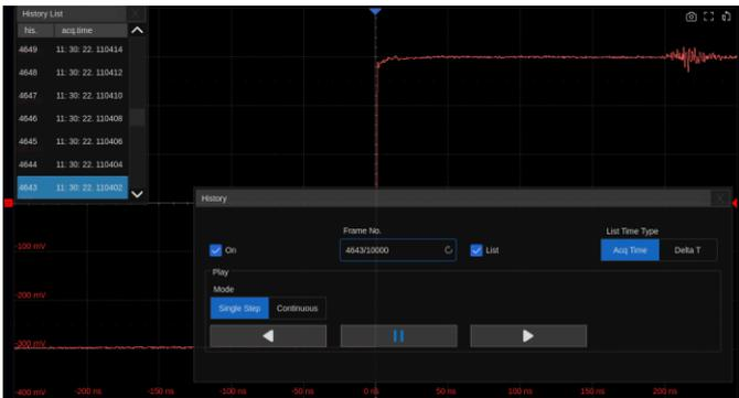
History function can record up to 170,000 frames of waveforms. The recording is executed automatically so that the customer can playback the history waveforms at any time to observe unusual events and quickly locate the area of interest using the cursors or measurements. The failed frames of the Mask Test can be stored as history
