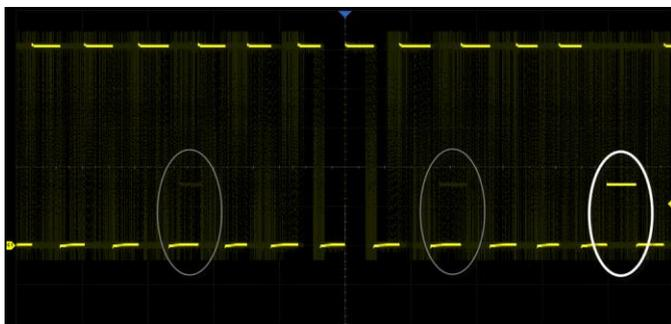
With a waveform update rate of up to 160,000 wfms/s, the oscilloscope can easily capture unusual or low-probability events. In Sequence mode, the waveform capture rate can reach 650,000 wfms/s
