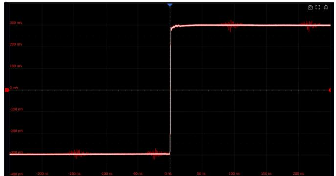
Segmented memory collection will store the waveform into multiple memory segments (up to 170,000) and each segment will store a triggered waveform as well the dead time information. The interval between segments can be as small as 1.5 μs. All of the segments can be played back using the History function
