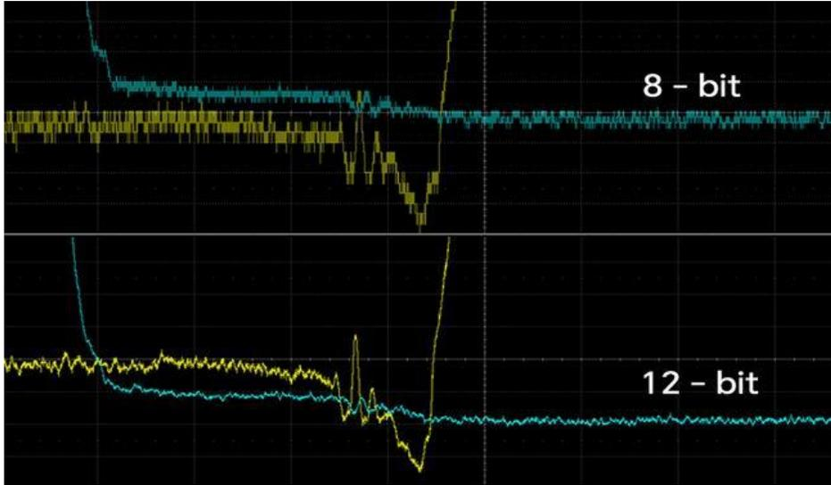
12-bit resolution shows you more details and less noise on the waveform.
