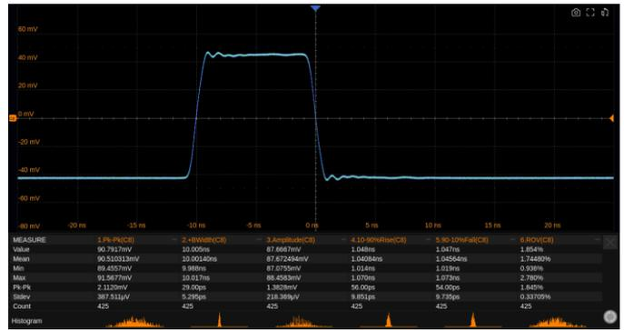
Statistics show the current value, maximum value, minimum value, standard deviation, and mean value of up to 12 parameters simultaneously. A histogram is available to show the probability distribution of a parameter. Trend and Track are available to show the parameter value vs. time.
